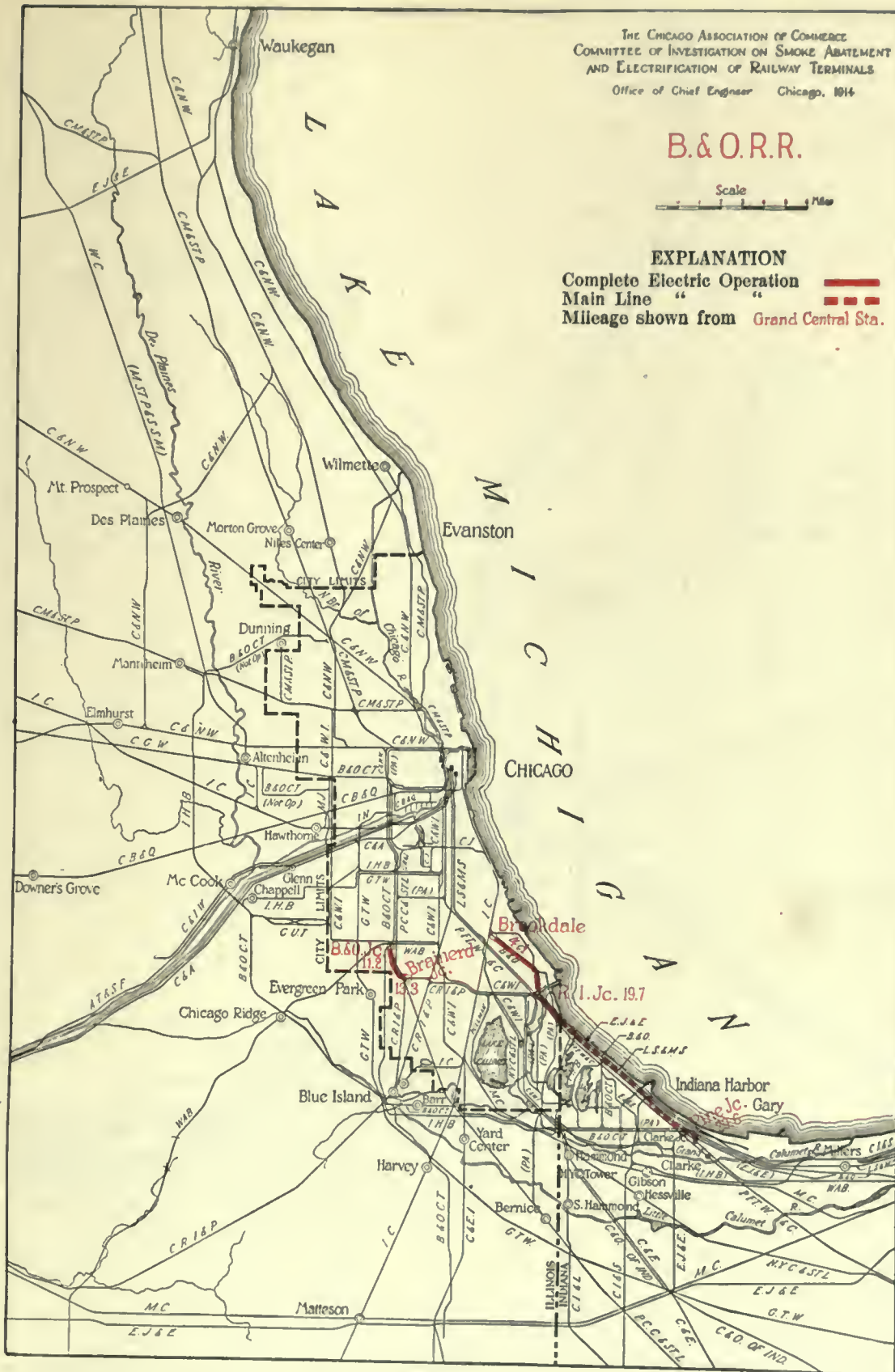
FIG. 545. TRACKAGE TO BE ELECTRIFIED BY THE BALTIMORE & OHIO RAILROAD
